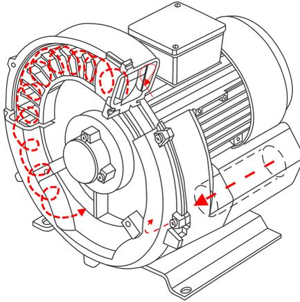
The machine works on the impulse principle, i.e. kinetic energy is transferred from the impeller to the conveyed medium and then is converted into pressure. The change in pressure is made without the use of any lubrication whatsoever.
